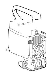
**5** Secure a cable with the cable clamp.
